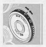
In special cases (flash, high filter compensating numbers over -3) the filter is compensated for by decreasing the film speed by 3° DIN for each full value (for example, when working with Neutral Density filter No.  $4:-4=4\cdot3^\circ=$  requires setting the meter to  $12^\circ$  DIN less than the actual film speed).
